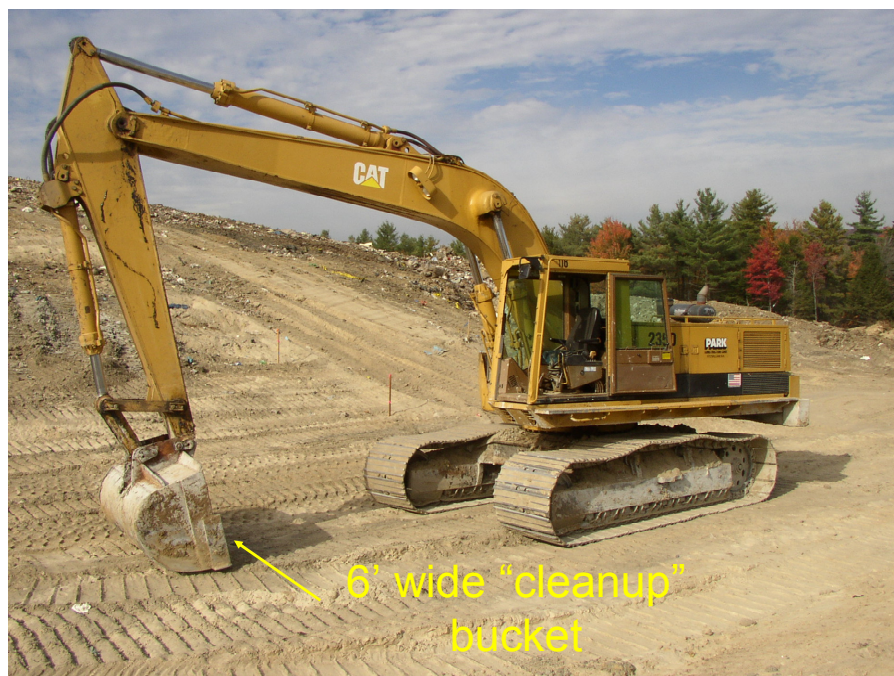
Figure 4.3 Trackhoe with 6-ft Cleanup Bucket
