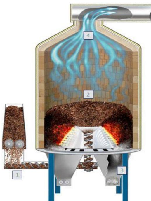
**Figure 1.** Gasification System. Description: (1) Fuel In-Feed System; (2) Gasifier; (3) Ash Removal; (4) Syngas [Source: Nexterra.]
