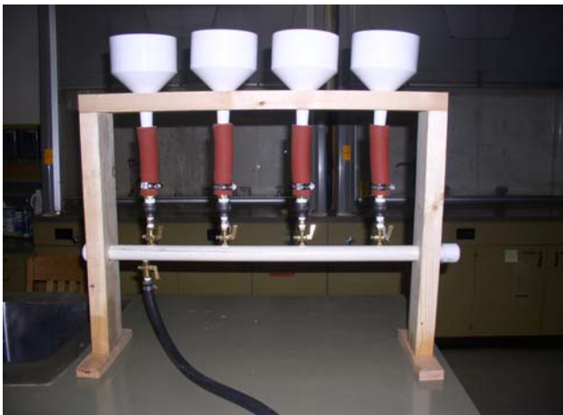
Figure 2. Vacuum filtration manifold with 4-110mm Buchner funnels.
