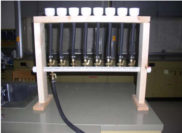
Figure 1. Vacuum filtration manifold with 8-55mm Buchner funnels.
