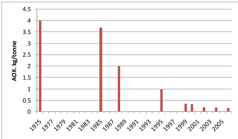
**Figure 5.3** Production-Weighted Mean Adsorbable Organic Halides (AOX) Discharges for U.S. Bleached Papergrade Kraft Pulp Production [See data explanation in text.]
