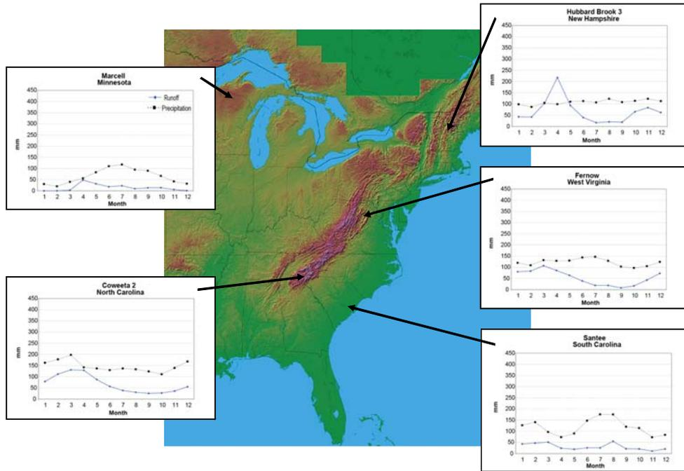
**Figure 3.2** Hydrographs (mm of water) from Research Watersheds across the Eastern U.S. Showing Different Patterns in Precipitation and Streamflow [Ziemer and Ryan 2000]
