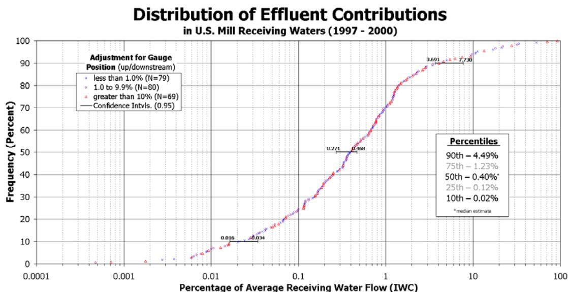
**Figure 5.4** Frequency Distribution of Instream Waste Concentrations as Percentages of Average Receiving Water Flows for U.S. Pulp and Paper Mill Receiving Waters, 1997 to 2000 [Beebe, Palumbo, and Eppstein 2003]
