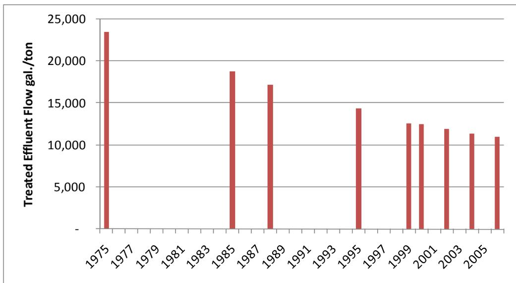
**Figure 2.2** Production-Weighted Mean Process Water Discharges for U.S. Pulp and Paper Production [see note in Section 5.1 concerning data shown]
