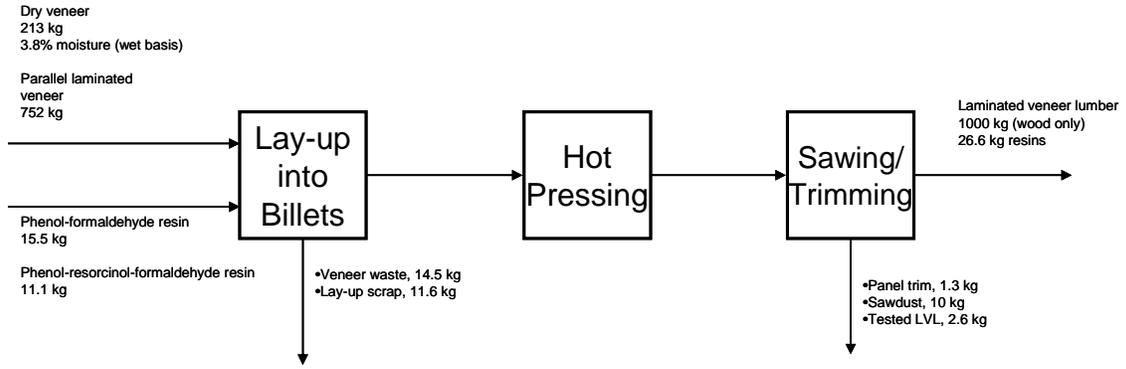
**Figure C.7** Laminated Veneer Lumber Mill, Weighted Average from 4 Facilities, wood(dry) mass balance [wood mass balance extracted from Wilson and Dancer 2005]
