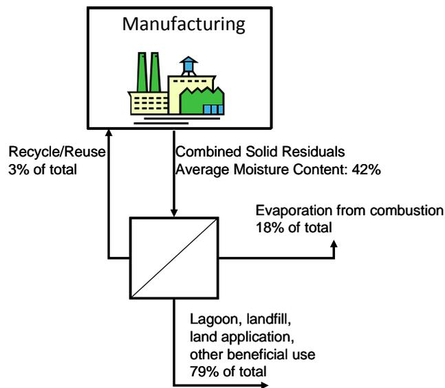
**Figure 4.5** Disposition of Water Contained in Solid Waste in the U.S. Pulp and Paper Industry
