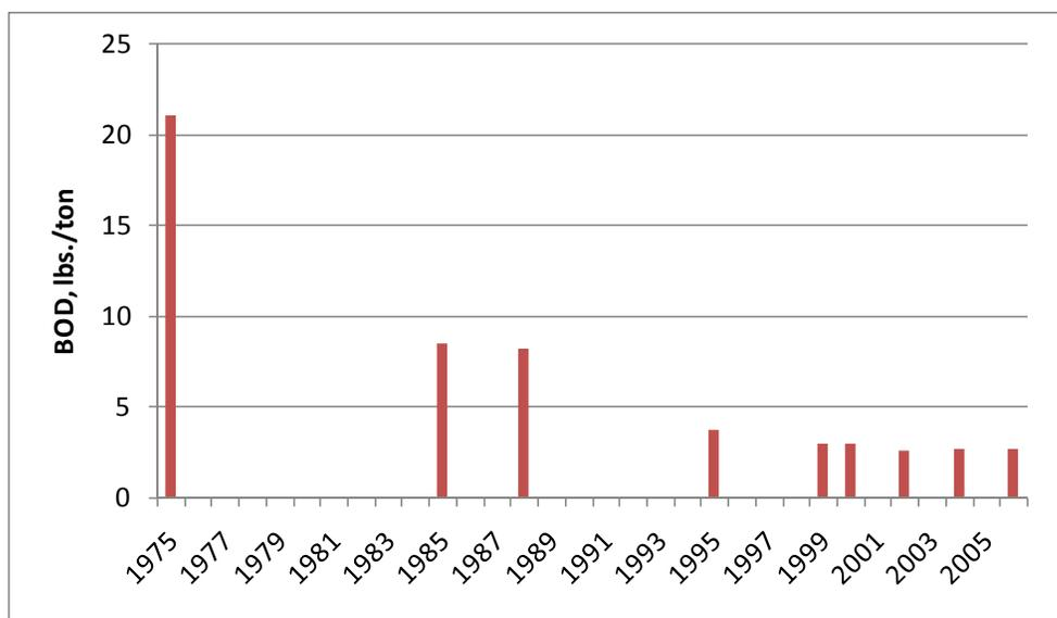
**Figure 5.1** Production-Weighted Mean Biochemical Oxygen Demand (BOD) Discharges for U.S. Pulp and Paper Production [See data explanation in text.]
