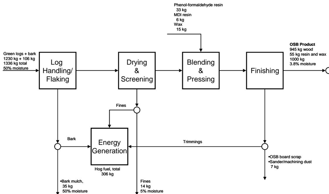
**Figure C.6** Southeastern Oriented Strandwood Mill Weighted Average from 4 Facilities, wood(dry) mass balance [wood mass balance extracted from Kline 2005]
