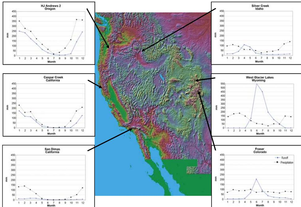
**Figure 3.3** Hydrographs (mm of water) from Research Watersheds across the Western U.S. Showing Different Patterns in Precipitation and Streamflow [Ziemer and Ryan 2000]
