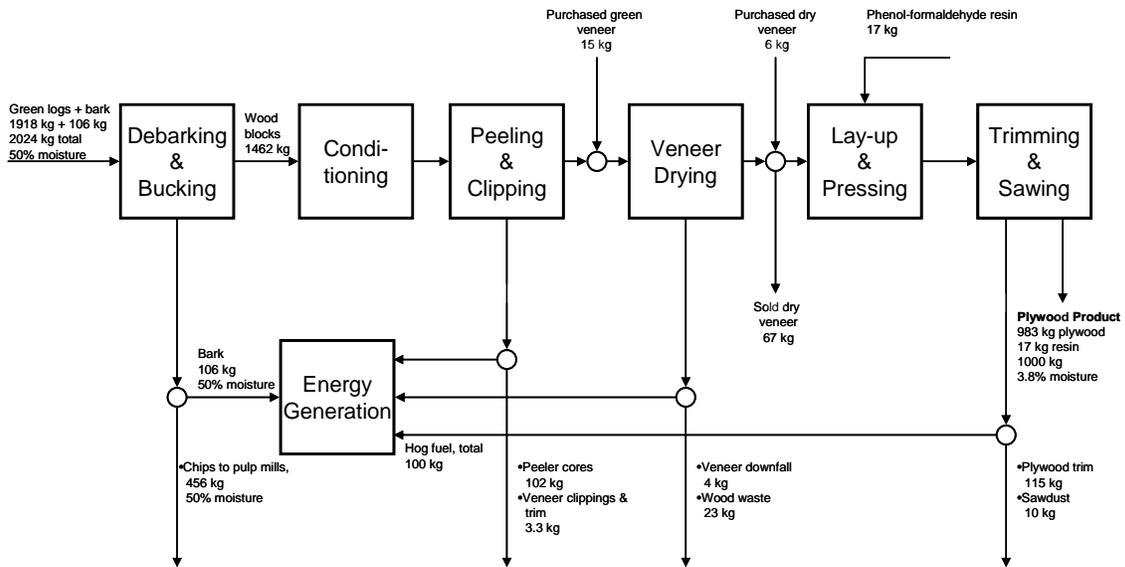
**Figure C.4** Pacific Northwest Softwood Plywood Mill Weighted Average from 5 Facilities, wood(dry) mass balance [wood mass balance extracted from Wilson and Sakimoto 2005]
