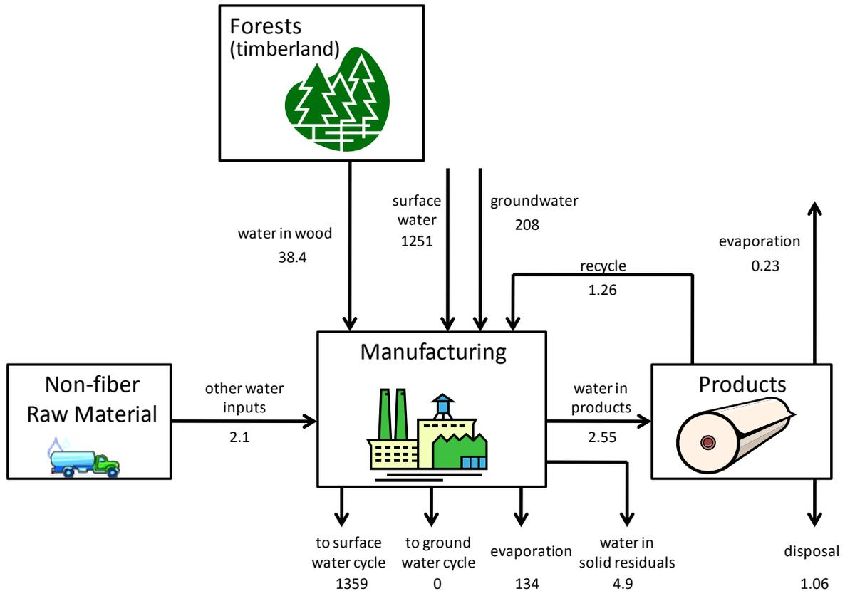
**Figure 4.1** Water Profile for the U.S. Pulp and Paper Industry (billion gal/yr)
