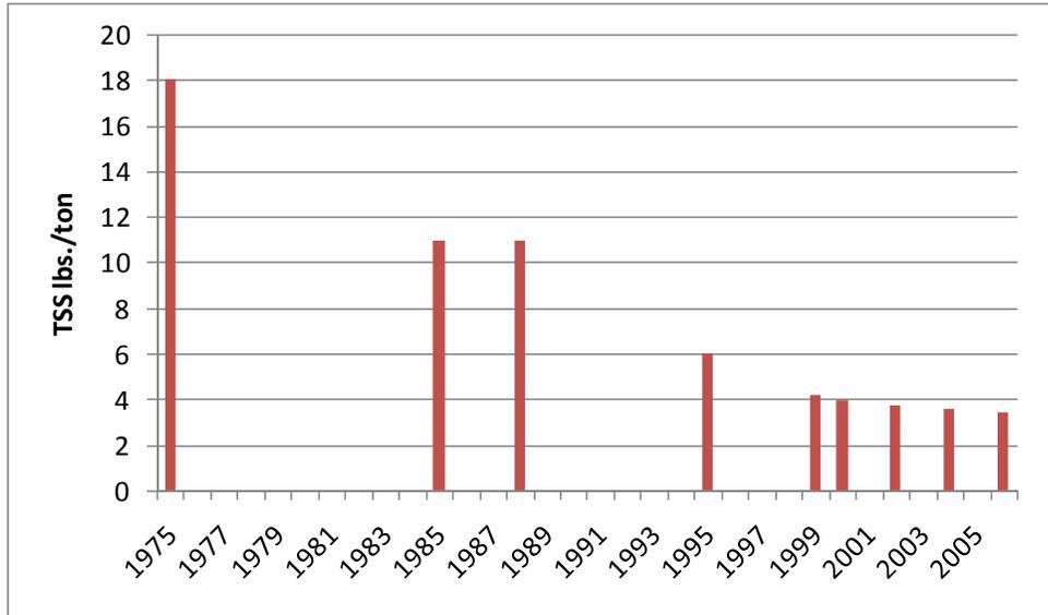
**Figure 5.2** Production-Weighted Mean Total Suspended Solids (TSS) Discharges for U.S. Pulp and Paper Production [See data explanation in text.]
