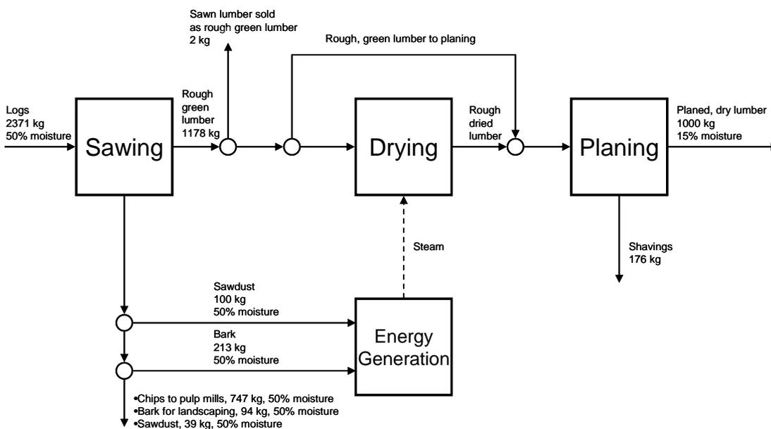
Figure C.2 Southeastern Softwood Lumber Mill Using Southern Pine [wood mass balance extracted from Milota 2004; Milota et al. 2004, 2005]
