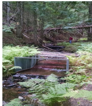
Photos: Flumes equipped with a pressure transducer and datalogger are often installed in long-term monitoring sites to quantify stream discharge. The flumes pictured here are located at Mica Creek Experimental Watersheds, Idaho.
