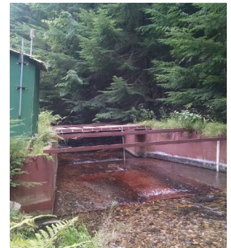
Photos: Flumes equipped with a pressure transducer and datalogger are often installed in long-term monitoring sites to quantify stream discharge. The flumes pictured here are located at Mica Creek Experimental Watersheds, Idaho.
