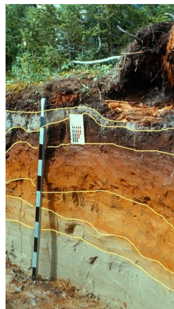
Figure 1: Dark colors indicate high carbon concentrations at the top of this forest soil profile. Climate, geology, forest type, and other factors affect how carbon enters, exits, and moves vertically and laterally within forest soils. Soil types differ in their properties and responses to disturbance, management, and other forces. Research and management that recognize these differences can provide place-based insights and practices that sustain soil carbon stocks while meeting other management goals.
