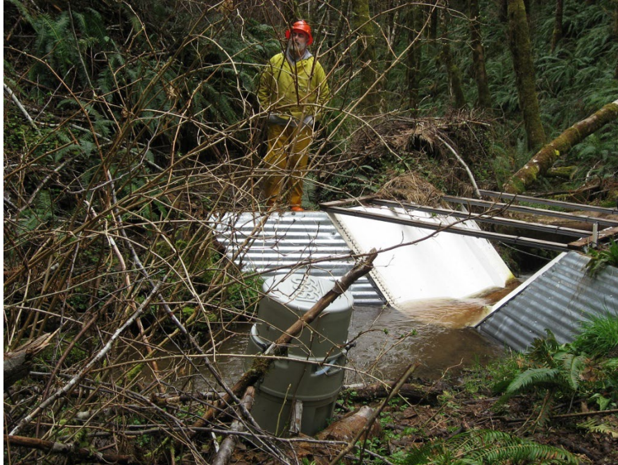
Figure B4. H-flume at NBH Gauging Station
