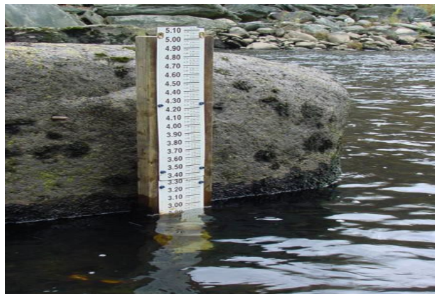
Figure B6. This Staff Gauge Reads a Stage Value of 2.92 Feet (Parker 2004)
